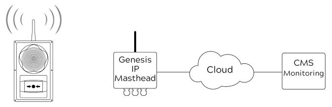
Silent test mode functionality is built in to minimise disruption and can be activated from any one of the NEXUS units using the key switch, or remotely when using an IP Masthead. A low battery alert is available when using the IP Masthead.
