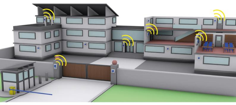
An IP Masthead can be added to the system so that up to 64 units can be monitored and controlled from one central location. This can be, for example, the site office computer or a Central Monitoring Station (CMS). Additionally, you can assign a name and location to each unit, ensuring a quick and efficient reaction to any alert event. You can also integrate with Immix and other popular CMS platforms.
