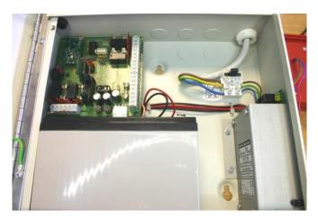
Fault' appears; check the connections and polarity. If the battery is connected incorrectly it is likely that the fuse will blow. The wiring should be corrected and the fuse replaced.
